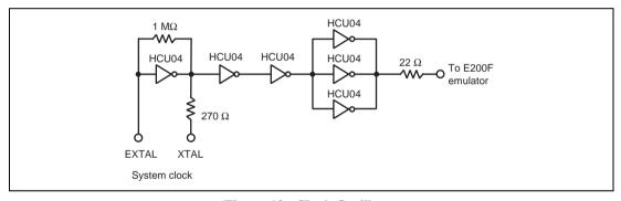
Figure 12 Clock Oscillator
